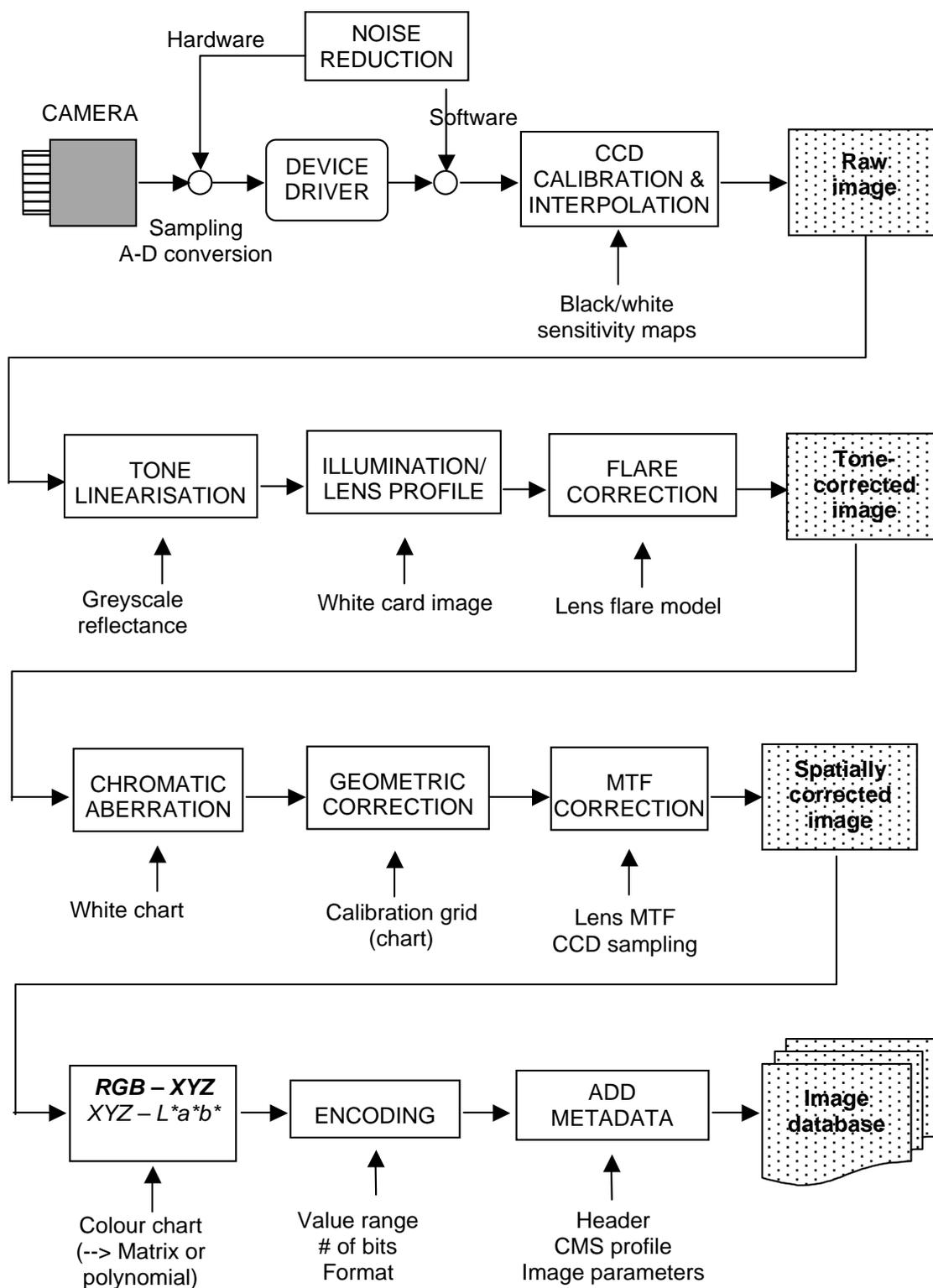
Figure 2: Sequence of operations in image processing chain.
