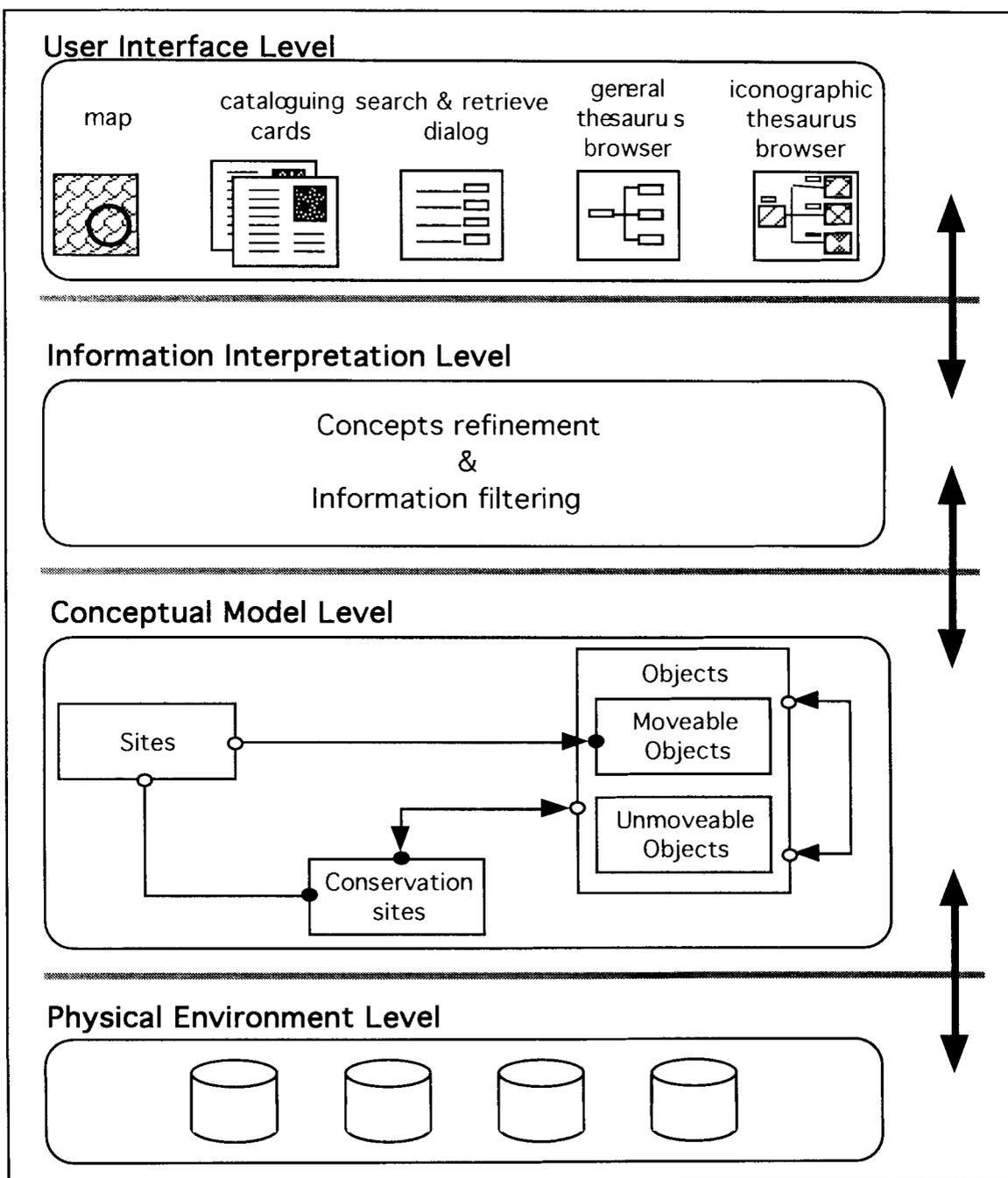
Figure 4 - The system architecture
