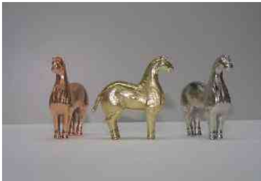
Fig. 9: Three physical replicas in plaster covered by metallic film electro-deposition. A pure copper statuette (left), a golden bronze (center) and a grey bronze (right)
