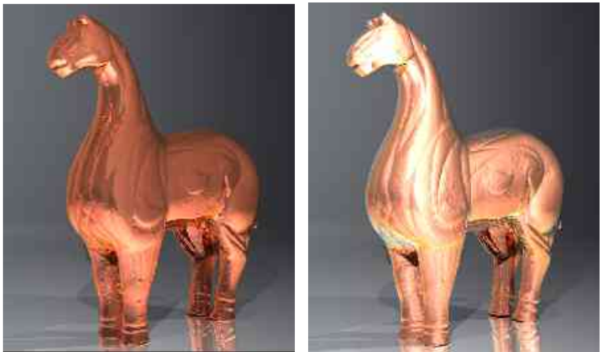
Fig. 8: A smooth surface of pure copper (left) and a moderately rough surface of pure copper (right), placed in the same lighting and viewing conditions. The rough statuette appears lighter due to the scattering of the incident and reflected light from the surface itself.
